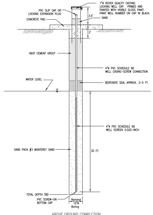
ABOVE GROUND COMPLETION DETAIL - MONITORING WELL (TYP.)
